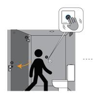
User enters and waves at 8606 (inside) to close the door. Door is automatically locked
