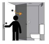
Janitor enters and twists the 8604/ 8605 (inside) back and forth when the door is open. The door will open to 90° and stop.
