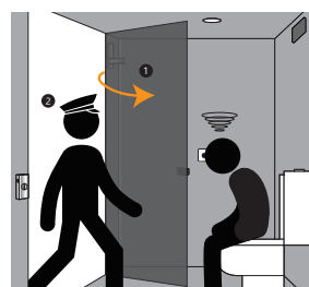
If no response from the user, the control room will unlock and open the door
