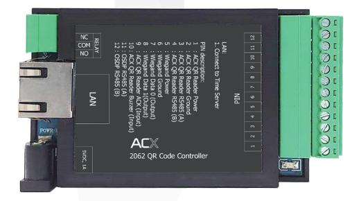
The ACX 2062 QR Code Controller works with the ACX QR reader series, the QR code controller can decode the ACX scramble QR code and the QR controller can output a fixed card number in wiegand or OSDP format.
