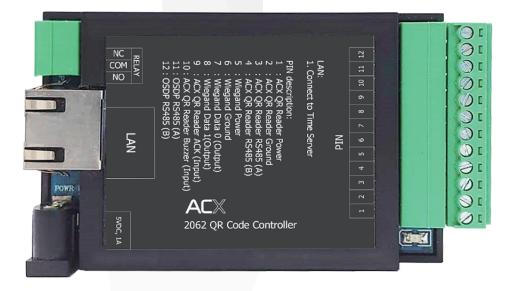
The ACX 2062 QR Code Controller works with the ACX QR reader series, the QR code controller can decode the ACX scramble QR code and the QR controller can output a fixed card number in wiegand or OSDP format.
